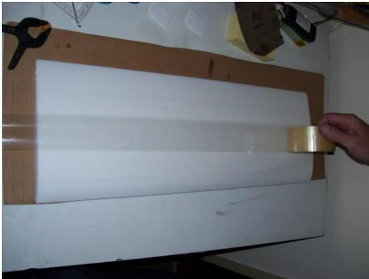
The following part is a little bit risky, but when applying correct it works just fine. Once the wing is covered, use the heat gun and cloth and heat up the packing
