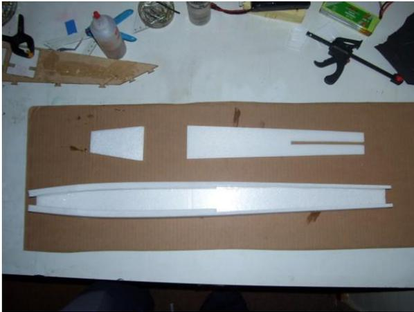
Glue the together with the fuselage, starting with the Front Section and then move to the rear section. Again, notice the 90 degree angle.
