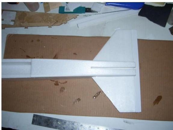
While you are busy with the elevator, locate the rudder (section C) and you can slot and glue that in place too.
