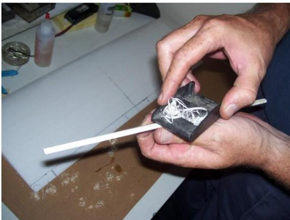
Sand/plane a 45 degree angle on the front side of the elevator. It allows much better movement for the elevator.
