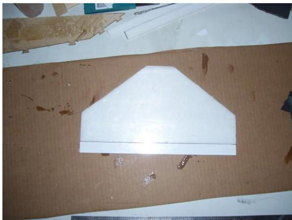
Trial fit the completed tailplane to the fuselage and if happy, glue it together, making sure it lings up properly with the wing.
