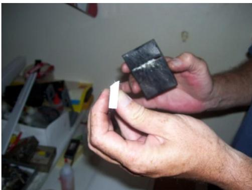
Put the 2 sections together to get the complete horizontal stabilizer. Use your favorite material to make the hinges. On all
